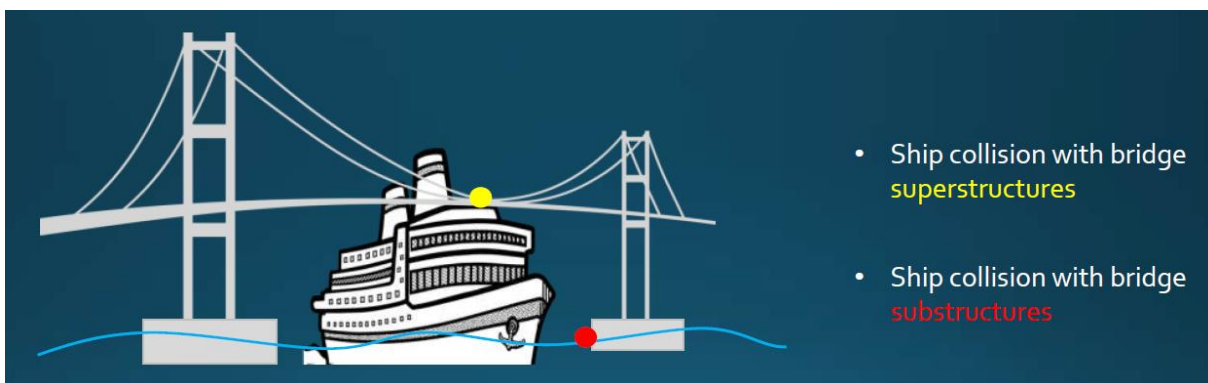
Figure 7: Collision to the substructures or superstructures. (Source: (Sha, Amdahl and Oiseth, no date))
